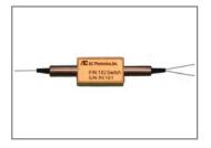
**ACP's** PMS Series switch connects optical channels by redirecting an incoming optical signal into a selected output fiber. This is achieved using a patent pending opto-mechanical configuration and activated via an electrical control signal. At the same time, the polarization state of the signal is preserved.
